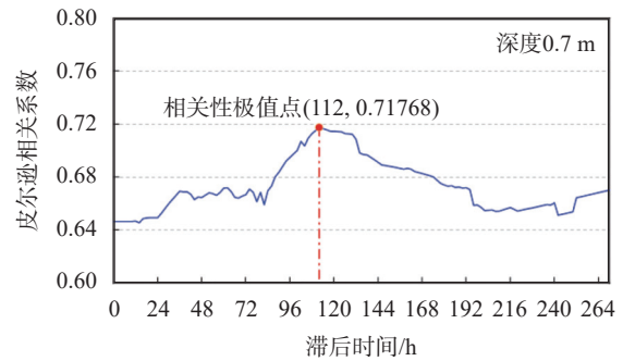
图 10 深度 0.7 m 土体含水率增量与降雨量的相关性及滞后性 Fig. 10 Correlation and hysteresis between soil moisture content increment at 0.7 m depth and rainfall
