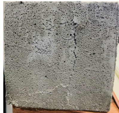
图 4 无侧限抗压强度下的 FFSS 破坏形态 Fig. 4 Failure modes of FFSS in the unconfined compressive strength test
