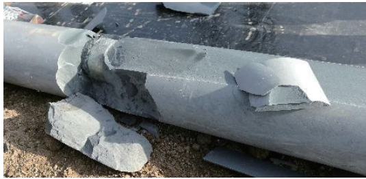
图7 锚固段无侧限张拉试验破坏
